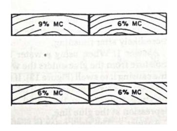
Planking can also occur when flat-sawn and quarter-sawn grain pieces are joined, as quartersawn piece shrink and swell twice as much as flat-sawn.
