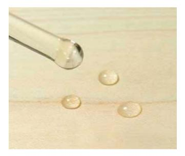
should disperse and get soaked into the wood within a minute or two. If the surface is inactive and will not be well attached to the glue, the water droplet will standup on the surface just like water droplets will appear on the hood of a freshly waxed car.
