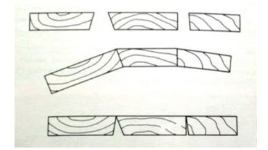
E. Opening of a miter joint. Miter joints are very sensitive to moisture content change. As a piece with a miter dries, it becomes more pointed, because it shrinks more in width than in length. Miter joints also have a lot of end grain; joints with a lot of end grain are not very strong unless splines or other techniques are used.
