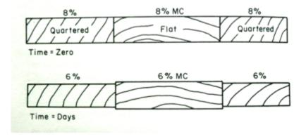
Planking can also occur when two dissimilar wood pieces are joined, as different wood products shrink differently than solid wood.
