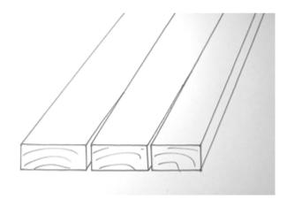
C. Planking. The third defect, which is often seen with a glossy finish, occurs when the individual pieces are at different MCs when assembled and then shrink or swell slightly as they adjust to their environment.
